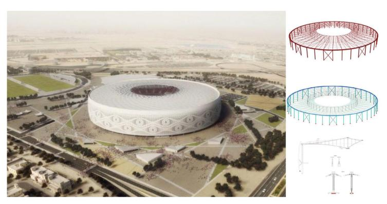
The use of advanced graphic and structural design tools (Grasshopper and Sofistik) helps to refine complex designs in which it is not always easy to assess the incidence of the various parameters involved. Parametric design facilitates a study of the different variants in order to properly understand the structure's overall behaviour and to find the optimal configuration.
